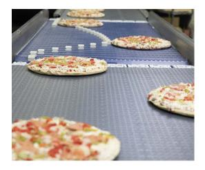
Active Integrated Motion<sup>™</sup> (AIM<sup>™</sup>) technology transforms frozen pizza handling by enabling automation in washdown environments.
