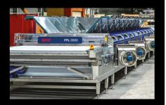
system with the hygienic qualities of a highly accessible, allstainless steel design, the tunnel has applications in both the confectionery and bakery industries.
