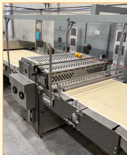
Dough travels through the rotary cutting station.
