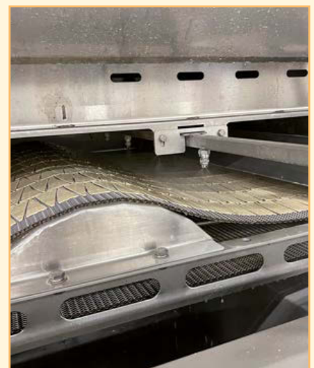
Rotary cut dough pieces pass through the cooler.
