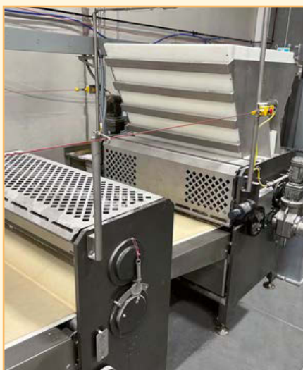
Dough feeds into a sheeter and 2 gauge rolls.
